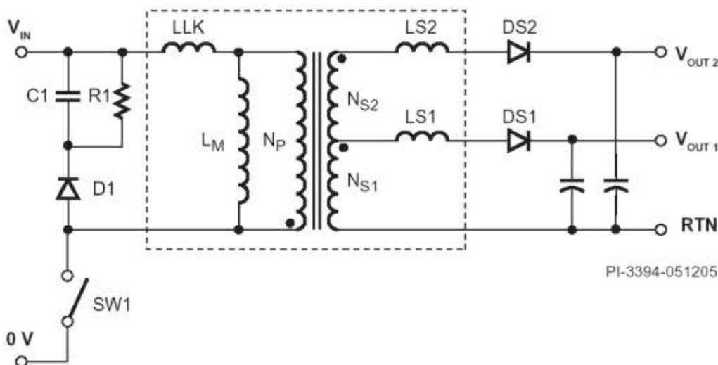
Figure 8 – Schematic of Transformer Model for a Multi-Output Power Supply
