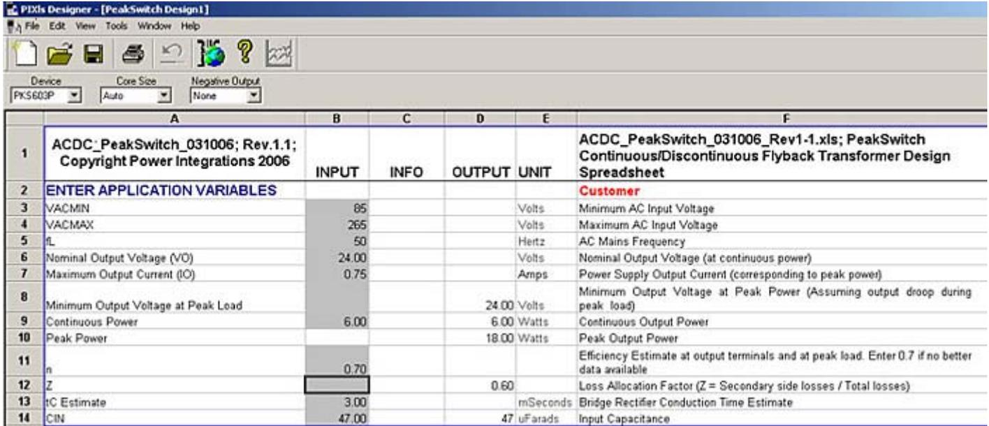
The screenshot shows a spreadsheet titled 'ACDC\_PeakSwitch\_031006; Rev.1.1; Copyright Power Integrations 2006'. The spreadsheet is organized into columns: A (Input), B (Info), C (Output), D (Unit), and E (Customer). The 'Z' factor is highlighted in the 'INPUT' column, with a value of 0.70. The 'Z' factor is defined as the Loss Allocation Factor (Z = Secondary side losses / Total losses).
