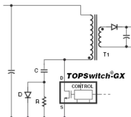
Circuit 'A' is a circuit that can be used either to clamp the drain voltage or to limit the rate of rise of the drain voltage at turn off.
