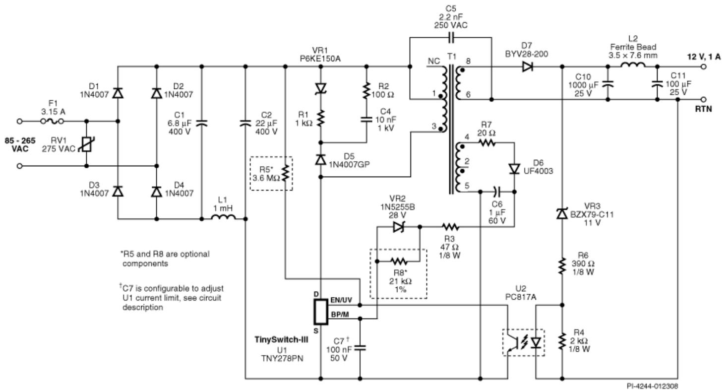
Figure 1. 12 W Universal input flyback power supply
