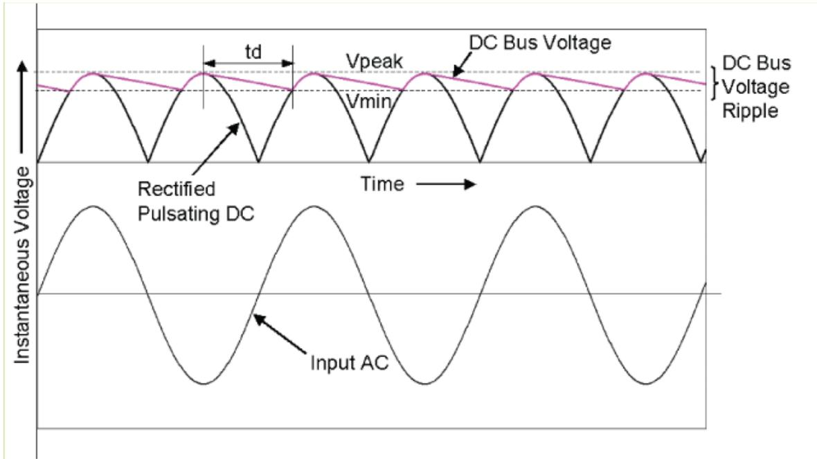
**Figure 2. Capacitive filter for full wave rectifier**
