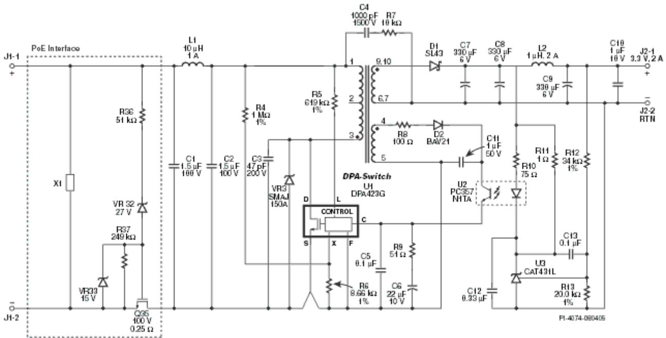
**Figure 1** – PoE Class 0 DC-DC Converter using DPA423G.
