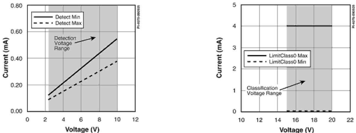
**Figure 2** – Class 0 - PoE Detection and Classification Specifications.
