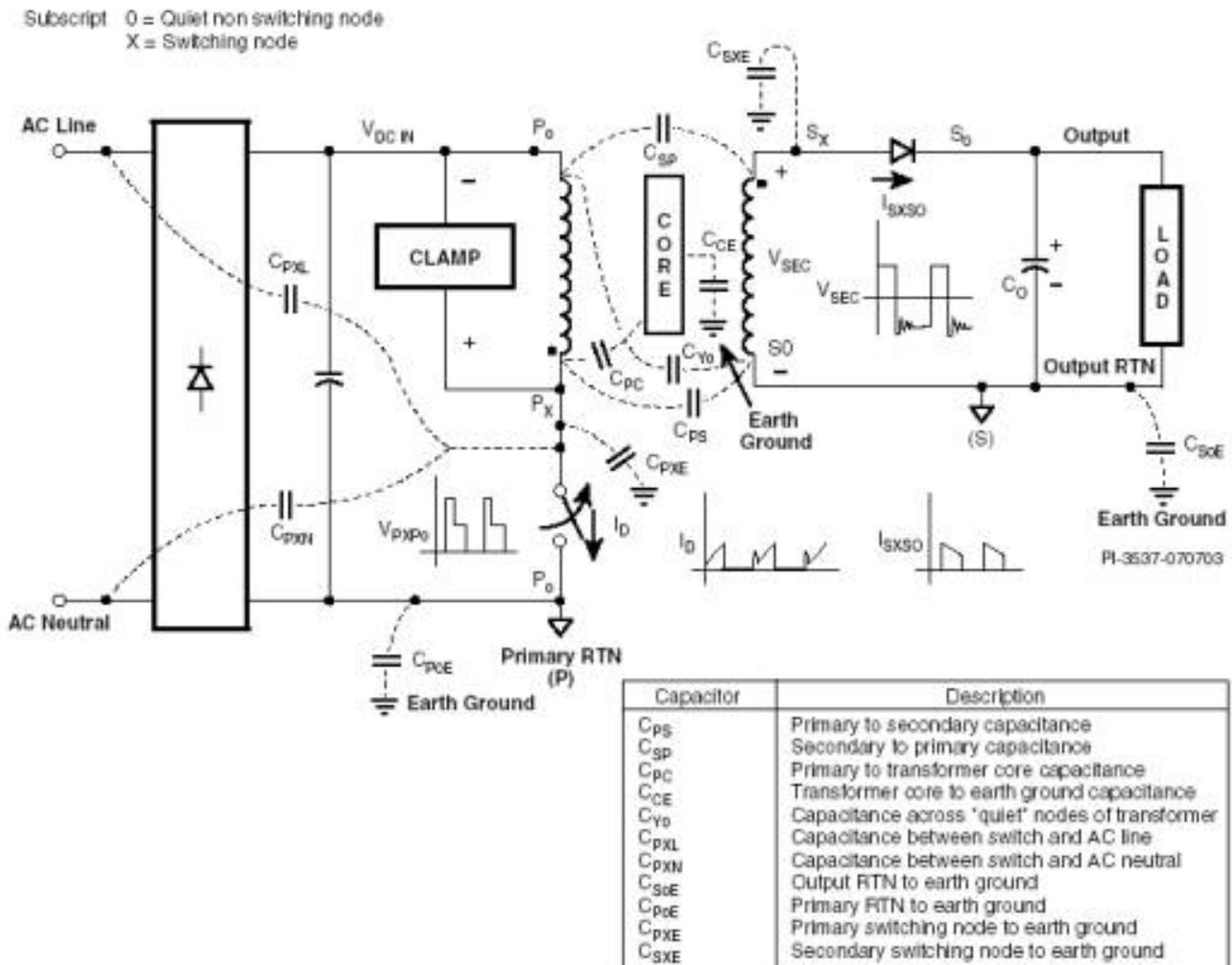
Figure 8 - EMI Sources and Coupling
