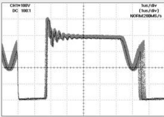
Figure 5 - TOPSwitch-GX Jitter Waveform
