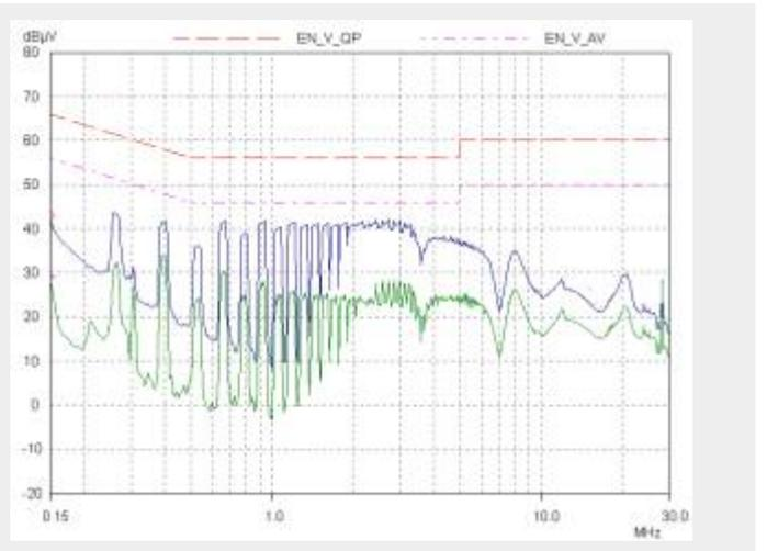
Figure 7 - TOPSwitch-GX (132 kHz) with jitter Conducted EMI versus Frequency
