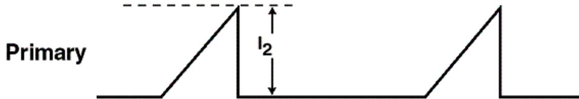
**Figure 2** - Primary Current - Borderline Continuous/Discontinuous,  $K_p \geq 1$
