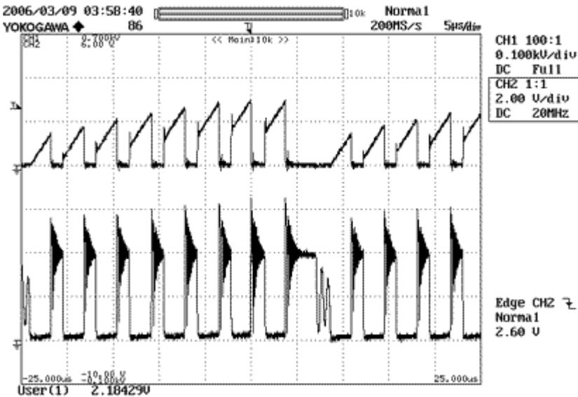
**Figure 2. Waveform shows Drain current (Top) and Drain Voltage (Bottom).**
