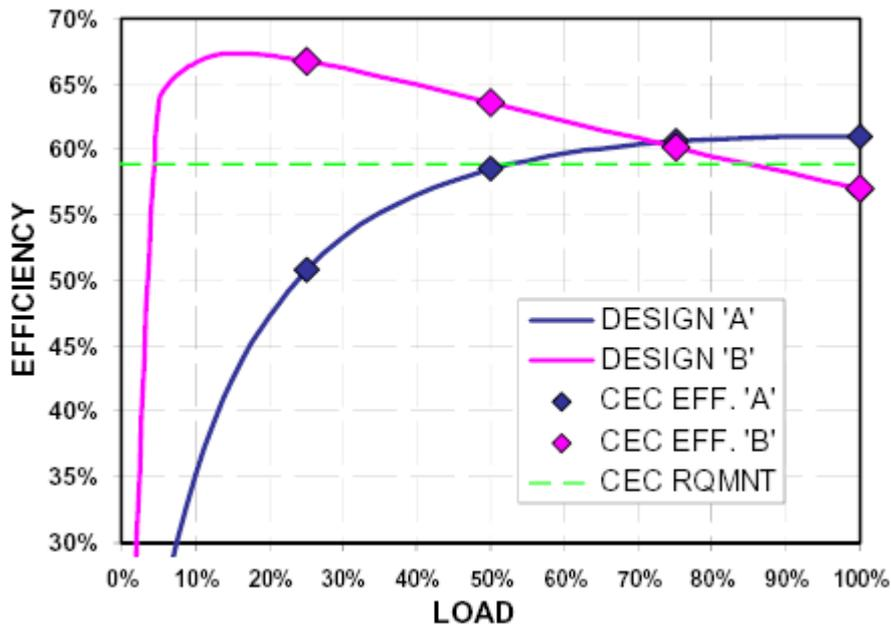
*TinySwitch-II* circuits can achieve such high light load efficiency because *EcoSmart*<sup>®</sup> technology automatically reduces the frequency of operation at light loads as a result of the On/Off regulation system, only switching to provide a power pulse when required. Consequently, switching losses are reduced to a minimum.
