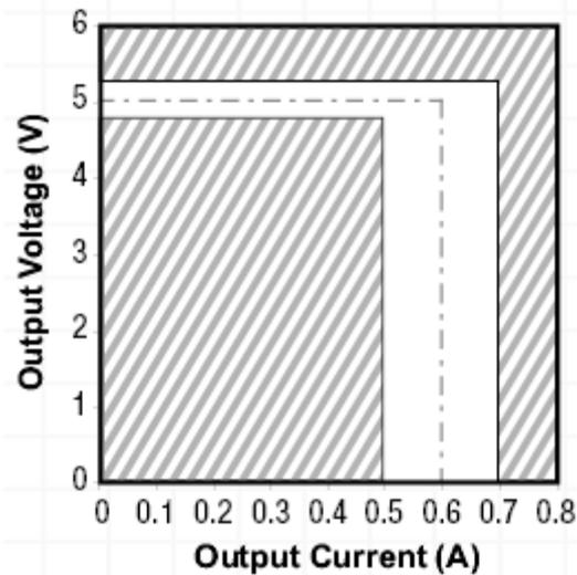
A 3 W, 5 V CV/CC charger requires the characteristics as shown:
