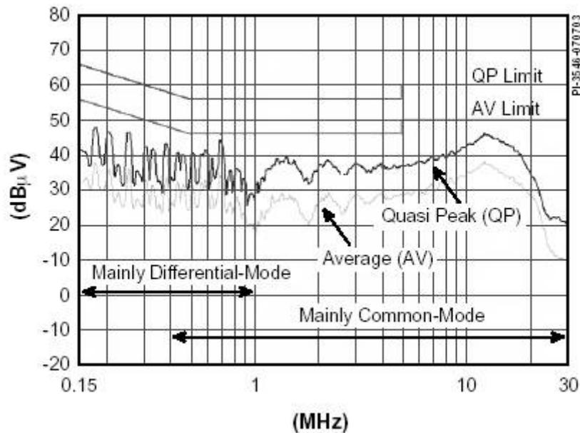
Figure 2 - Portion of Frequency Spectrum showing areas of Differential Mode and Common Mode Noise
