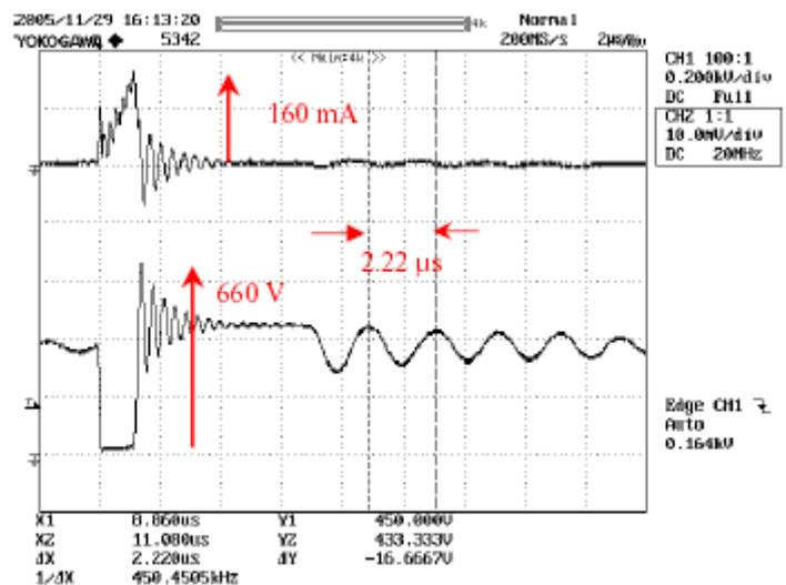
Drain Voltage and Current (200 V, 100 mA, 2 μs/div.)
