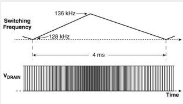
Figure 3 - TOPSwitch®-GX Jitter Frequency
