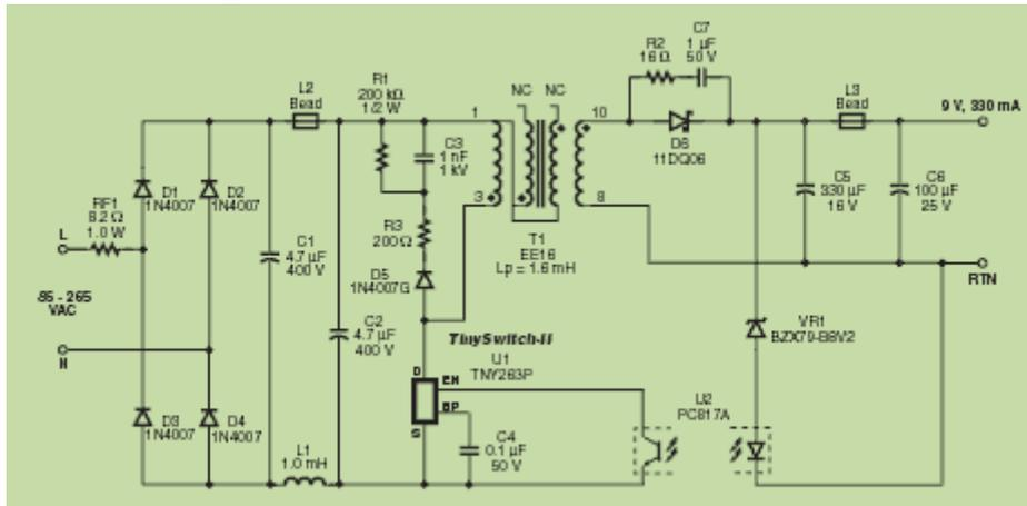
The schematic to the right shows a typical Flyback AC-DC power supply delivering 3 W and utilizing a TNY263P power conversion IC.
