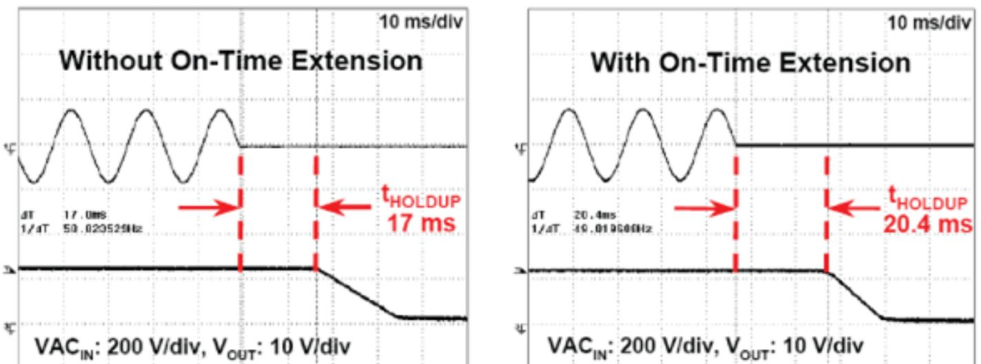
**Figure 6. Improvement in hold up time with on time extension**
