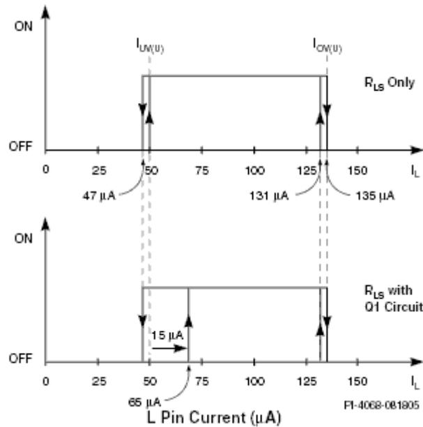
**Figure 5** - Circuit for Modified Under-Voltage (UV) Turn-on Threshold with Hysteresis (approximately 10 VDC in this case).
